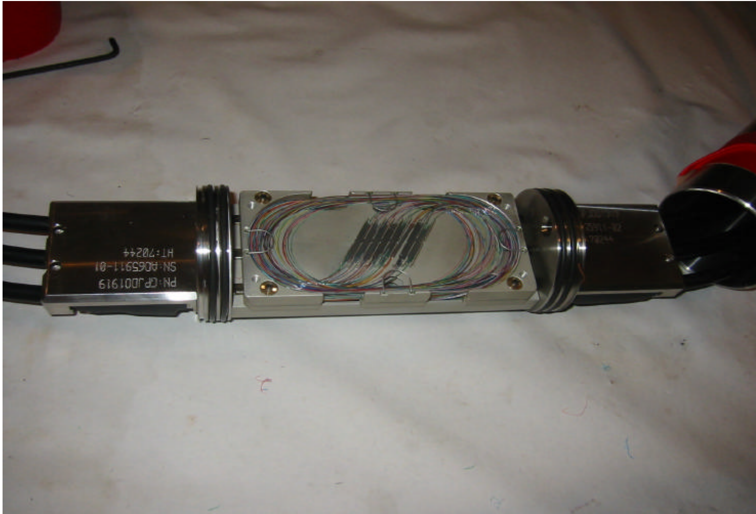
3 off FO ELEMENT JOINT BOX FOR HYBRID AC POWER CABLES
