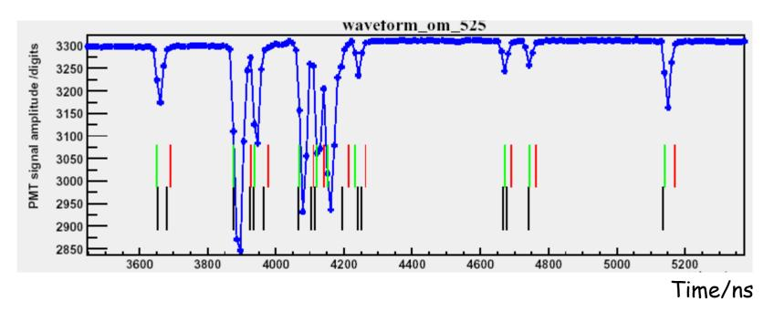
Very complex structures of multi-photon hits not measured by the old DAQ Need for pattern recognition and appropriate likelihood models -> in work
