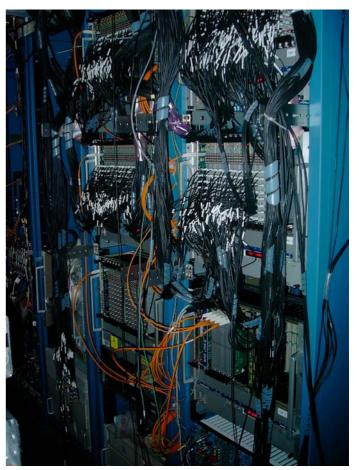
100 MHz FADC, 12 bit, (Struck)
